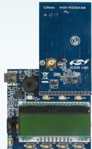
EZRadio® Si4010/Si4355 ONE-WAY AES DEVELOPMENT KIT
